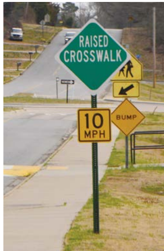
Raised crosswalks induce traffic to slow down, and are helpful for child safety near schools.
