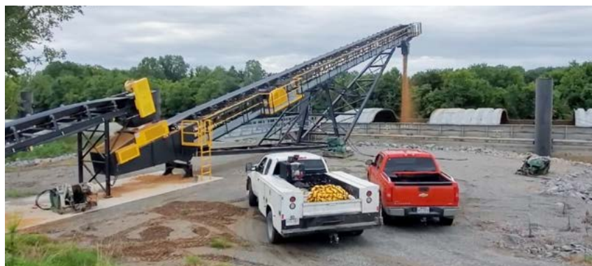
The Little Rock Port Authority continues to expand multi-modal freight capacity and capabilities. The direct rail/truck to barge conveyor system funded by an FY2016 TIGER grant is the latest system to be put to use. Photo credit: Little Rock Port Authority.
