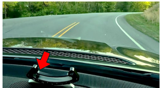
Figure 14: RSA team's ball bank indicator maxed out at 19 while driving southbound on Batesville Pike at 35 mph around the curve north of Greer Road.
