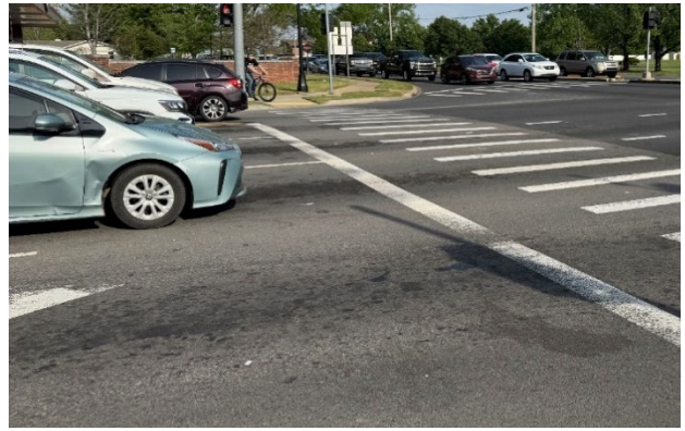
Figure 29: Visibility for right-turn vehicles at the southbound approach of South Donaghey Avenue to Dave Ward Drive is limited by a brick wall at the northeast corner of the intersection.
