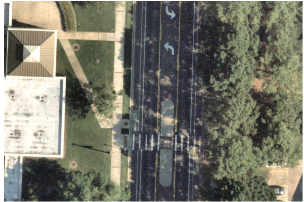
Figure 14: Sidewalks connecting the University of Central Arkansas PBS building to the sidewalk along the west side of South Donaghey Avenue do not align with the RRFB crossing.
