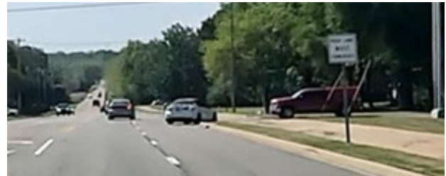
Figure 31: Right lane must turn right sign posted for southbound right-turn lane for University Park Apartments Driveway is posted in advance of Moix Boulevard, where cars were observed turning right.
