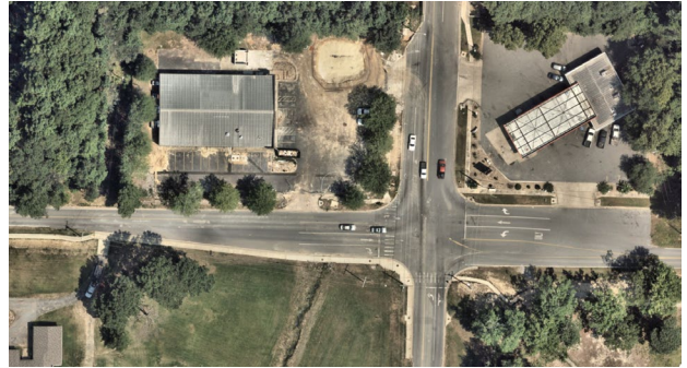
Figure 16: Aerial of the intersection showing lack of pavement markings as approaches widen to provide dedicated turn lanes.
