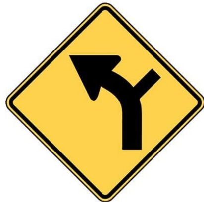
Figure 30: MUTCD intersection within curve warning sign W1-10L that should be considered for this location.
