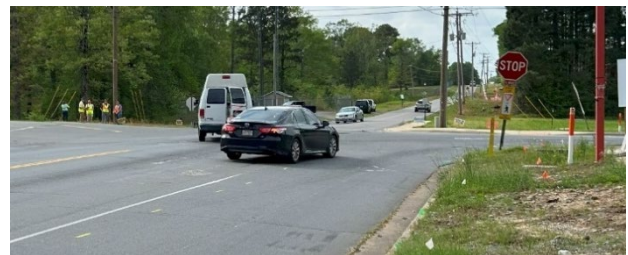
Figure 15: Vehicles observed turning right onto Pleasant Hill Road from the shared left-thru lane of southbound Vimy Ridge Road (where there are no in-lane arrows or stop bar pavement markings).
