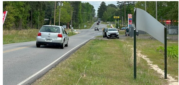
Figure 13: Faded pavement markings along Vimy Ridge Road and no lighting present south of Loganberry Drive.
