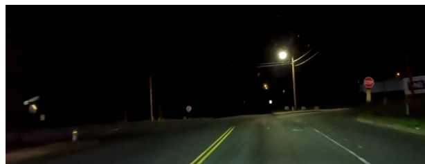
Figure 8: A single light exists at the southwest corner of the intersection of Vimy Ridge Road and County Line Road and does not provide sufficient lighting to illuminate the entire intersection.
