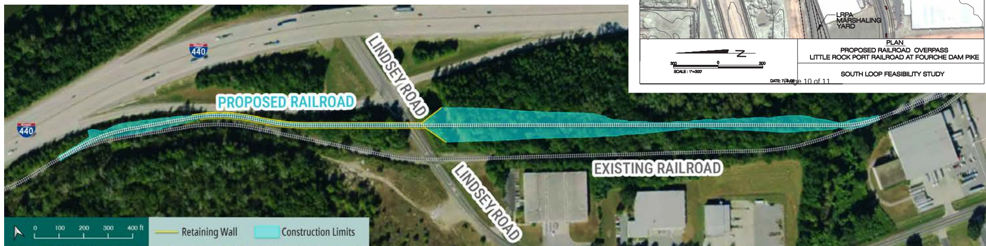
FIGURE 16: GRADE SEPARATION OVER FOURCHE DAM PIKE
