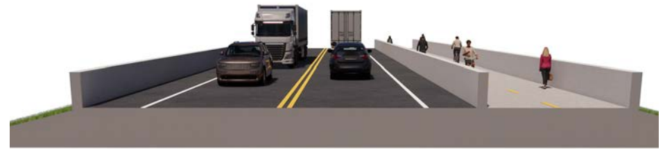
Two-Lane Bridge with Sidepath
