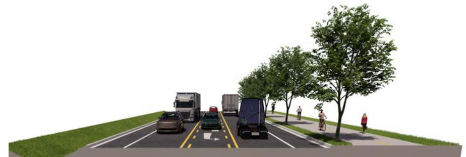
Three-Lane with Sidepath or Sidewalk
