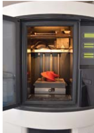
The 3-D printer (at left), and Len Hill, founder of NAMJet, shows a prototype impeller blade, produced in the printer.
