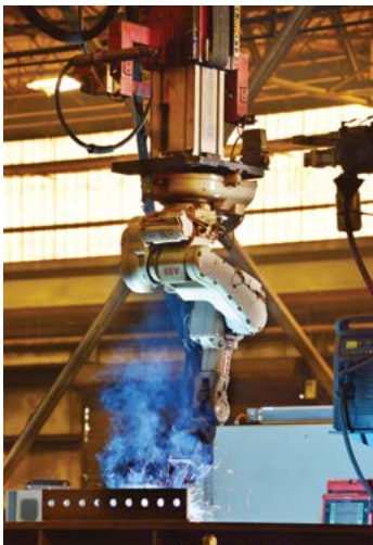
A robot welder has sped up the process and reduced production costs.
