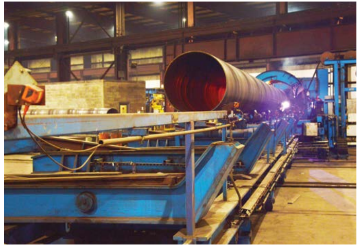
The glow shows where the newest segment of pipe is being cut from a continuous production run.
